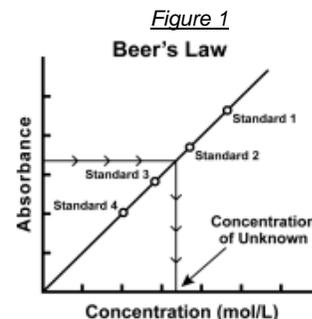
You will determine the concentration of an unknown  $\text{CuSO}_4$  solution by measuring its absorbance. By locating the absorbance of the unknown on the vertical axis of the graph, the corresponding concentration can be found on the horizontal axis. The concentration of the unknown can also be found using the slope of the Beer's law curve.
